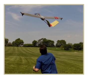
The EP-2000 is a tough, survivable, fixed-wing sensor platform designed for missions covering long loiter times. Emphasis has been placed on stability and ruggedness. Principal applications include: precision agriculture services, public utilities applications, and emergency response, and search and rescue missions. The EP-2000 is a custom designed aircraft that can be tailored to user requirements.
